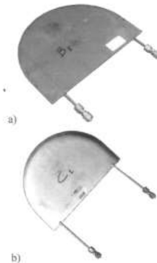
Fig. 1. Types of tested flat jacks. a) Jack B1; Jack C1.
