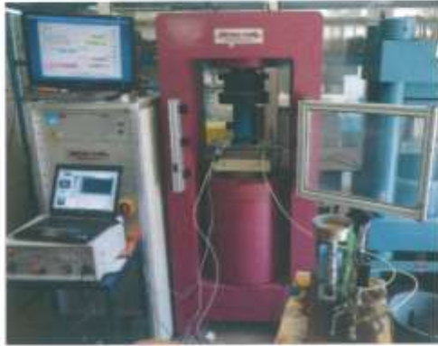
Fig. 3. Test on a flat jack.
